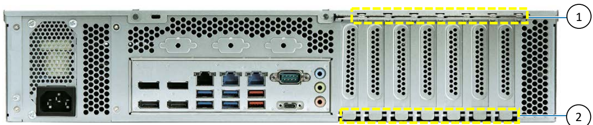
Figure 19: Installing Low Profile Expansion Cards
