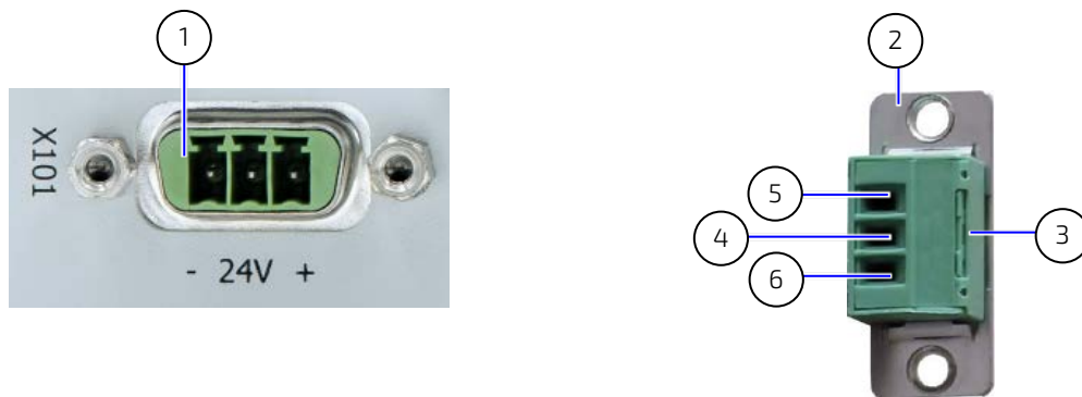
Figure 17: Power IN Connector and Mating Power Connector
